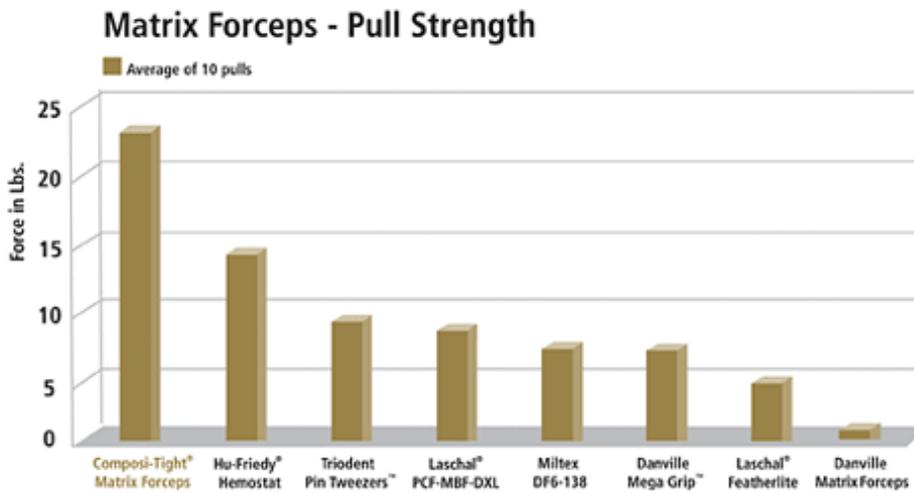
Testing was performed using a pull force gauge with .0013" matrix material. Each forceps was tested for 10 pulls, with the average force shown in the chart below.
